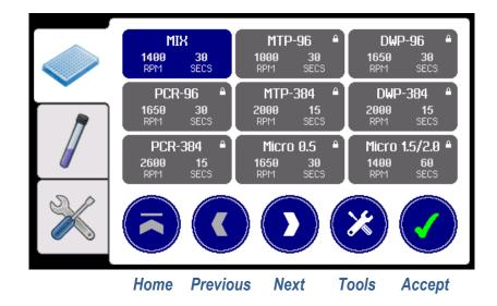
Each program grid button shows the program's ID and the assigned speed and time parameters.
