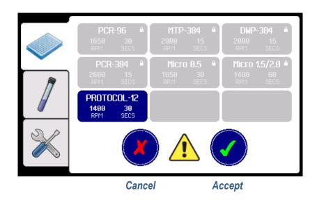
Next press the Accept button to confirm the deletion, or Cancel to exit.
