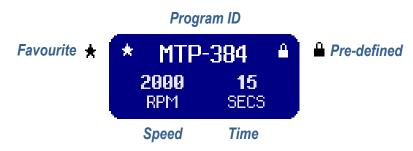
To load a program, use the **Home** button to jump to the top of the program grid list or the **Next** and **Previous** buttons to scroll through the list to highlight the desired program, and then press the **Accept** button.
