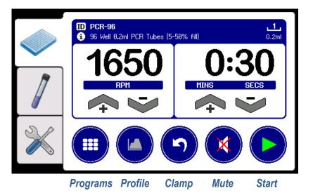
The adaptor block type is displayed in the top right-hand corner of the status area, or as 'x' if none is required. Refer to sections 6.3.3 and 6.3.4 for details relating to the use of specific adaptor blocks.
