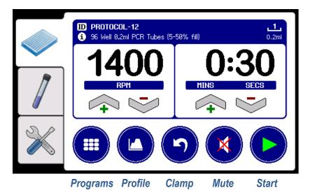
Once **Unlocked**, the **Increase** and **Decrease** buttons can be used whilst the mixer is running to fine tune the mixing performance for the particular plate type, sample solution and fill volume being used. Any changes to these parameters are automatically saved to memory for next time.
