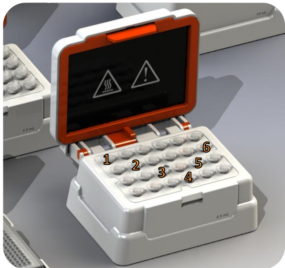
Figure 3: Details of the positions of each thermocouple within and around the Heated Module
