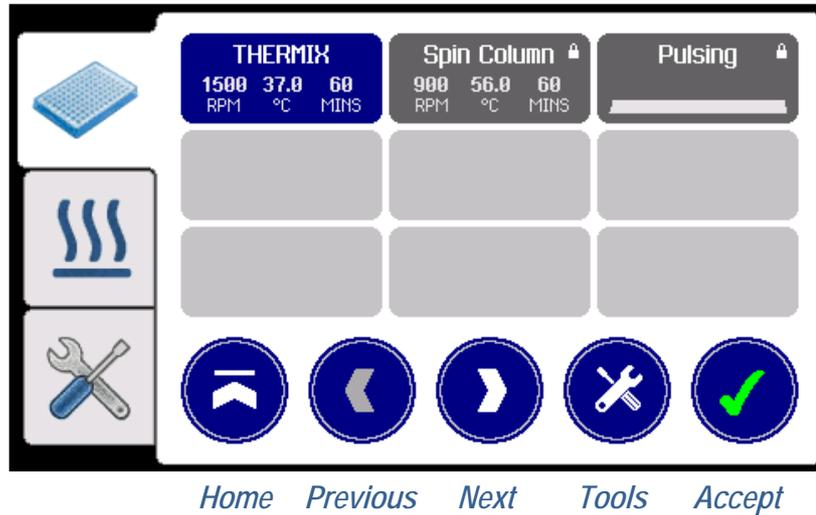
**i** If a Heated Module is attached, it will automatically select the program that it most recently ran. Hence, when swapping between modules, each module remembers the last program it used.
