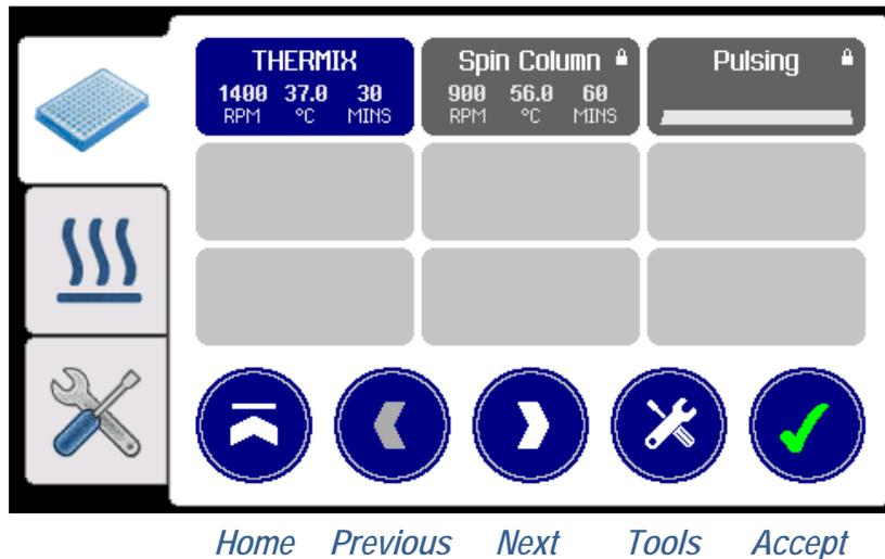
To load the **THERMIX** program, first attach a Heated Module to the unit, then select the **Mixer** page tab, and press the **Home** button, followed by the **Accept** button.
