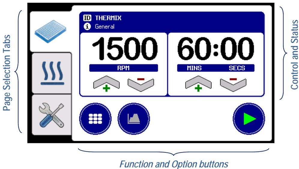
The Ther-mix is designed to allow simultaneous mixing and heating of sample plates and tubes, by providing easy display mode switching using the three page selection tabs shown in Table 4.
