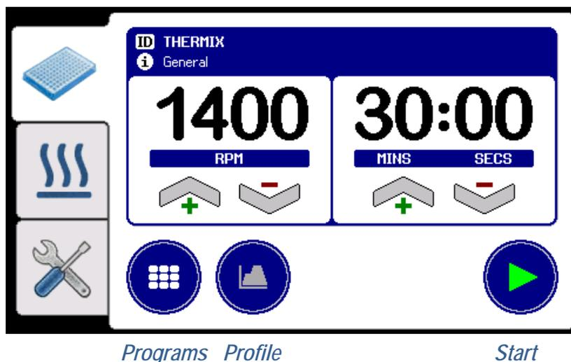
The block and lid heaters will also be switched on at this point and begin to control to the specified temperature set points. The progress can be checked, or the set points modified, by selecting the **Heater** page tab.
